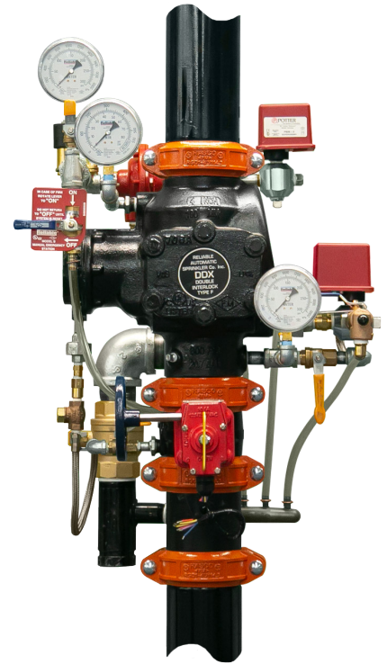
Figure 2. Modern deluge valves can be trimmed for use as deluge systems, preaction systems, and dry pipe systems. In some cases, the same valve can be used to create 11 types of systems (Reliable DDX Type F Double Interlock System).
