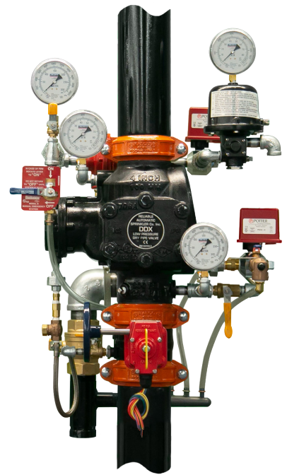
Figure 1. Today’s mechanical style dry pipe valves are deluge valves trimmed to make them operate as dry pipe valves. In essence, the loss of system air or nitrogen pressure becomes the detection event (Reliable DDX-LP).
